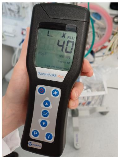
Figure 4: Hygiena SystemSure Plus ATP luminometer used for ATP measurement.
