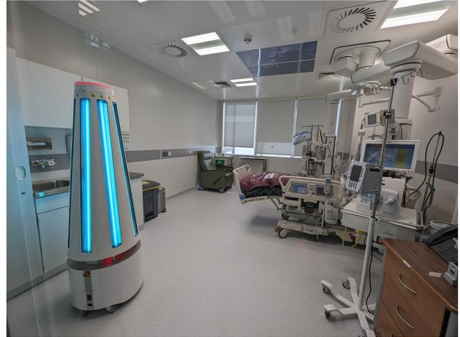
Figure 1: Omnia UV-C disinfection robot in room ICU1.
